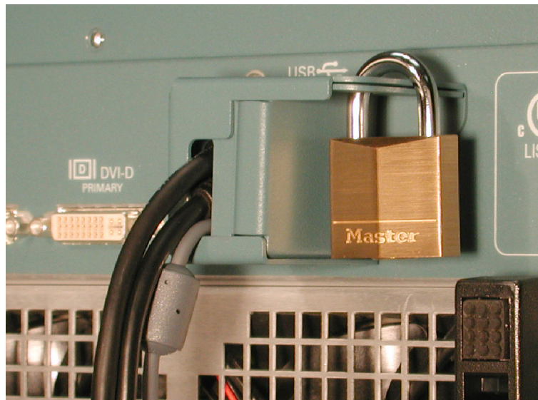
Figure 5-9: Attach a padlock
