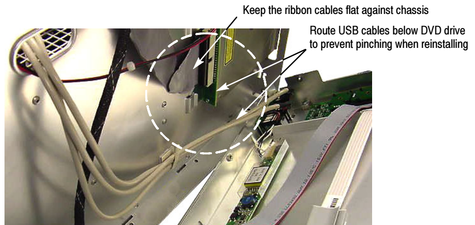
Figure 5-5: Dress the cables properly
